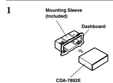
Slide the mounting sleeve into the dashboard.
